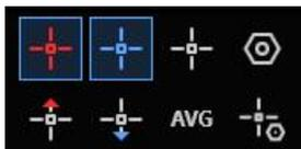
① Cursor tracking
