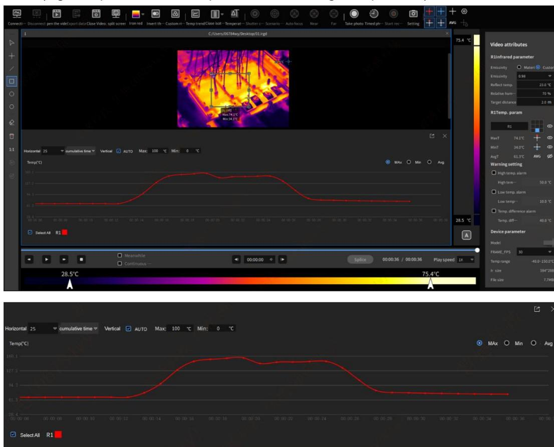
① Left click: click the curve, and the temperature values will be displayed at the sampling points of the time-temperature curve for intuitive display of the temperature values at the sampling points.
