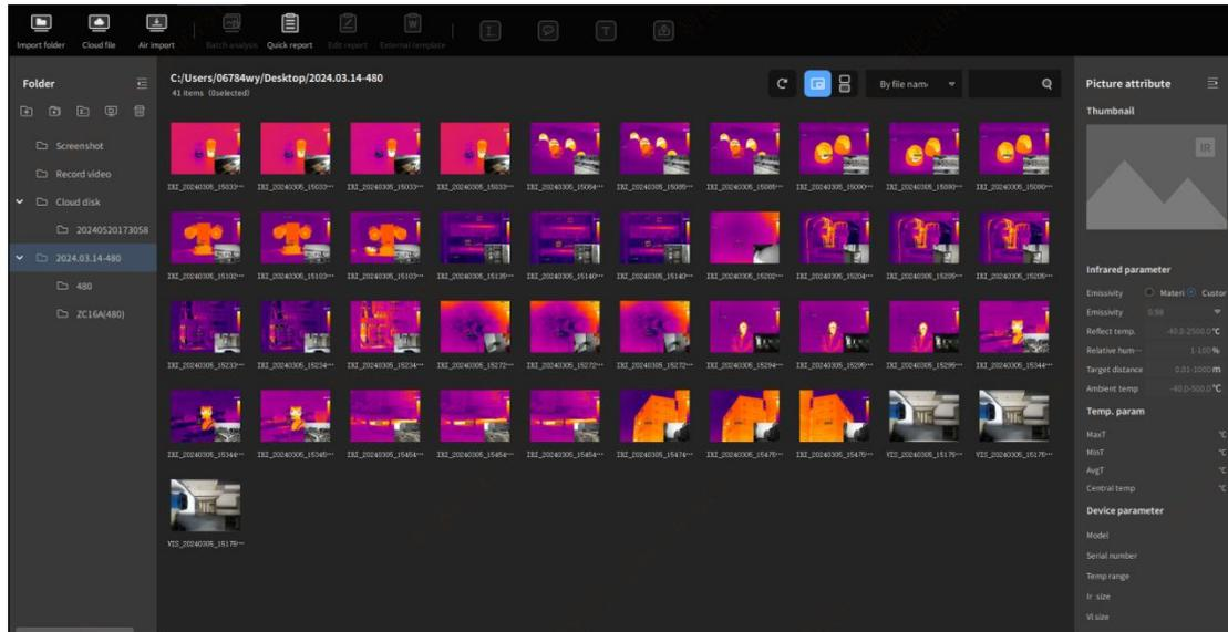
Classify and manage the infrared thermal image or video files stored in the computer. Batch analysis of thermal images and batch export of reports are available.
