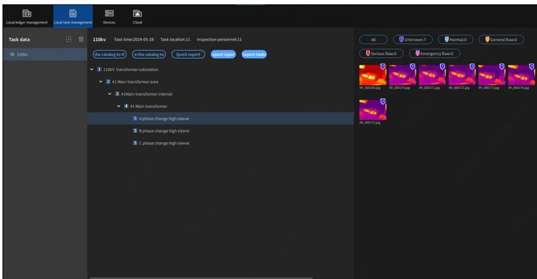
7. Conduct image analysis in the ledger or task module, and create inspection path batch reports.
