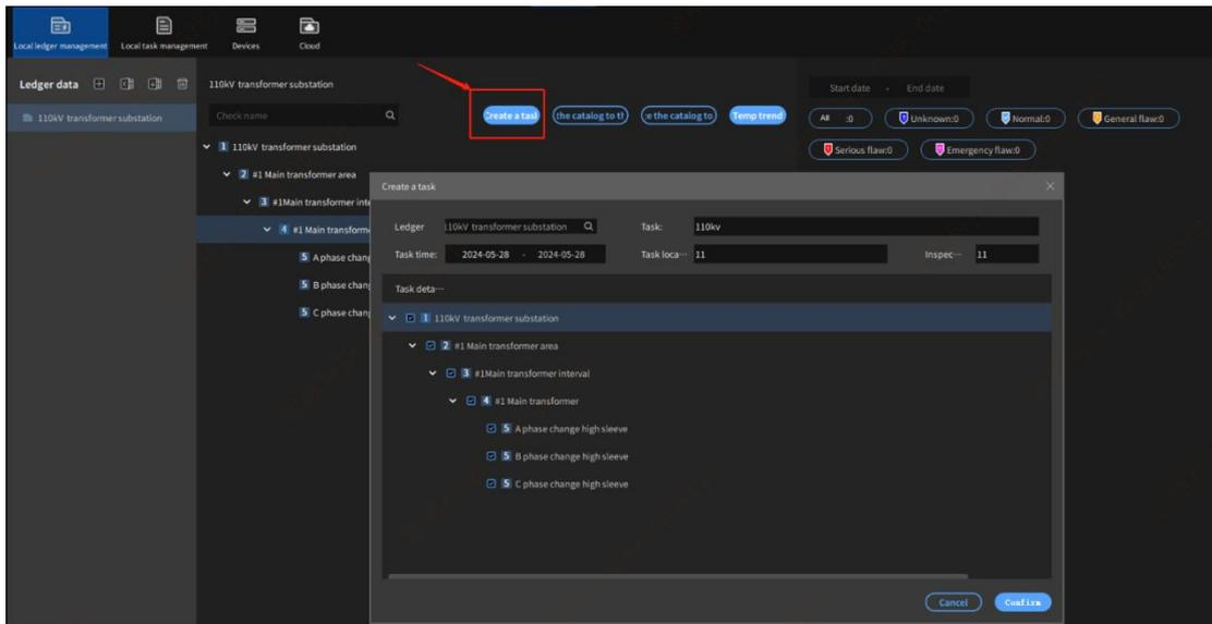
4. Synchronize the local inspection task on PC to the infrared thermal imaging camera or interact with the existing ledger task system.
